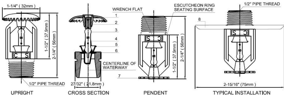
1.SSU DEFLECTOR 2.SET SCREW 3.GLASS BULB 4.FRAME 5.BUTTON 6.SPRING SEAL 7.SSP DEFLECTOR 8.STANDARD ESCUTCHEON
